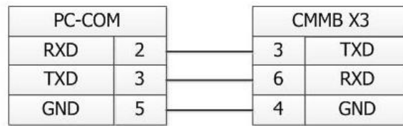
Figure 0-3 DSub 9 of PC and X3 of driver
